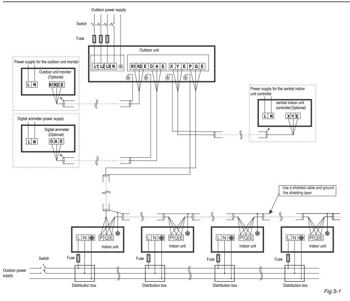
280/335 Three-phase electrical control system connection of the outdoor unit
