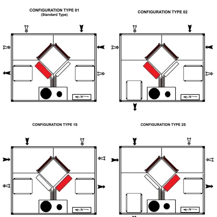
The air intakes can be layed in-line or at 90° by changing closing panels each other.
