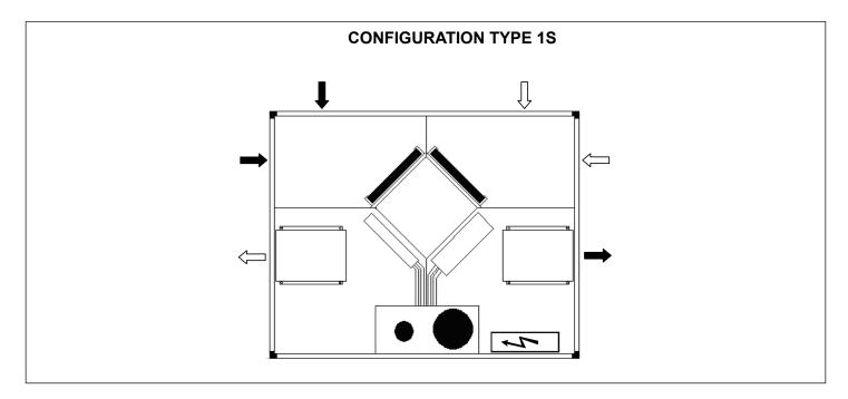
The air intakes can be layed in-line or at 90° by changing closing panels each other.
