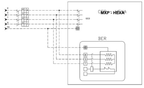
Dashed lines show the connections to be carried out by installer
