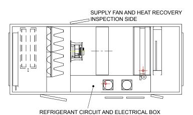
**KEY** Pre-filter and fine filter on fresh air 1 2 Filter on return air intake 3 Thermal wheel heat recovery 4 Supply fan 5 Exhaust fan 6 Condenser-evaporator 7 Evaporator-condenser 8 Compressor 9 Bioxigen module 10 Electric or water additional heater Built-in electrical board 11
