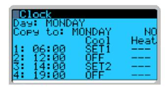
It is possible to copy the current day setting to other days by using the function "copy to:" that copies the current daytime settings to the target date in the "copy to:" line
