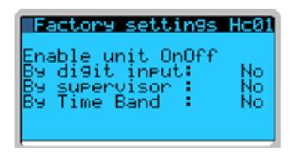
At this point it's possible to command the input unit (see circuit diagram for the connections) or by time bands. Pay attention that only after you enable the previous procedure will be able to see the pages that allow setting time bands.
