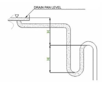
Connect the discharges from each condensate collection pan to the sewerage system either directly or via the manifold.
