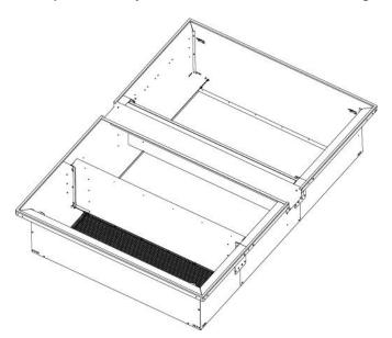
Example of adjustable roofcurb without condensing
