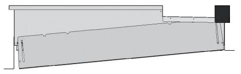
After levelling the frame, secure the adjustable returns on the trimmer.
