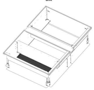
Example of non-adjustable roofcurb with condensing unit
