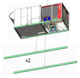
The surface must support continuously the entire area of these 2 rails (no rubber pad, no spring, no block...). See bottom view of the unit:
