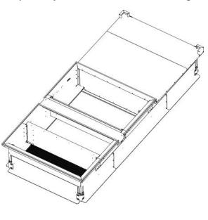
WARNING: all the roofcurb must be strongly secured to the ground
