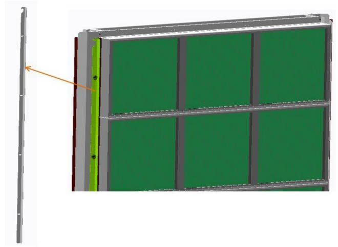
Use this stop to slide the dirty filters out one by one into the rail.
