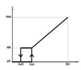
Modulation and ON/OFF H51=1(factory set) Voff = H52 = 0,5V (factory set) Von = H52 + H53 = Voff + H53 = 0,5+0,5 = 1V
