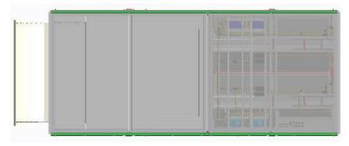
In case of installing the unit on dedicated structure (for example a specific metallic frame structure), the structure must be compliant with the unit base frame design and dimensions (width is the same for all units; length depends on the unit so refer to 2D drawing available):
