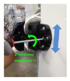
During this operation, it's important to keep a constant peripheral clearance (4mm) around the panel:
