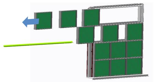
Replace the dirty filters by clean ones (respect the airflow direction).
