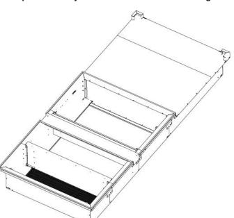
Example of adjustable roofcurb with condensing unit
