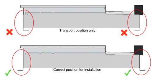
Place the roof mounting frame on the trimmer beam by first lining up the inlet and the outlet opening.
