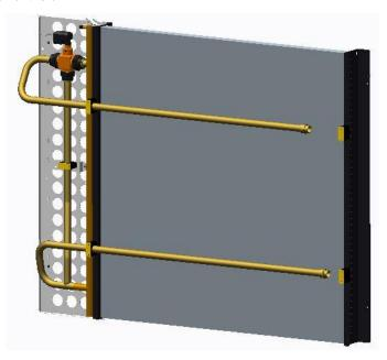
The freeze protection is made via fresh damper safeties nevertheless a full freezing protection has to be done using glycol.
