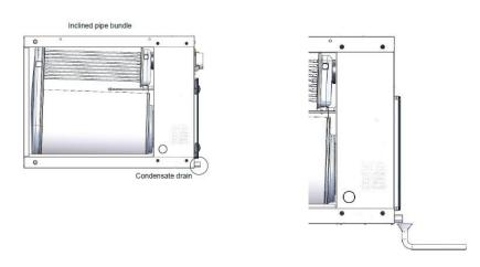
WARNING: Do not forget to connect the condensate drain (No need to add a siphon). The condensates must absolutely be drained at least 5 meters from the unit into an appropriate place/evacuation. The condensates are corrosive and could damage the unit (or other parts of the installation) if they are not drained properly.
