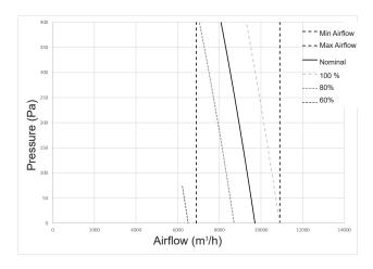
The curves show the adjustment for the nominal airflow. Other regulations are possible to reduce or increase fan performances.
