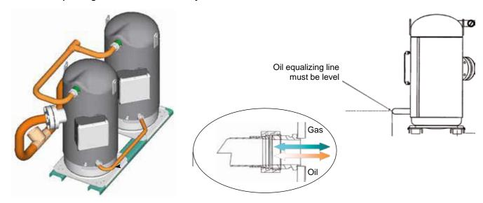
The oil equalizing Line is fitted with a sight glass which can be used to check the oil level in the compressor assembly. It is mandatory to stop both compressors to get a good reading of the oil level in the crankcase of the compressors.
