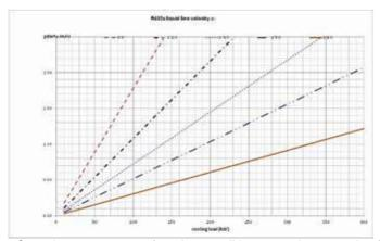
(2): at 45°C with 5°C subcooling and 8°C suction temperature; for other conditions, use the correction factor table.
