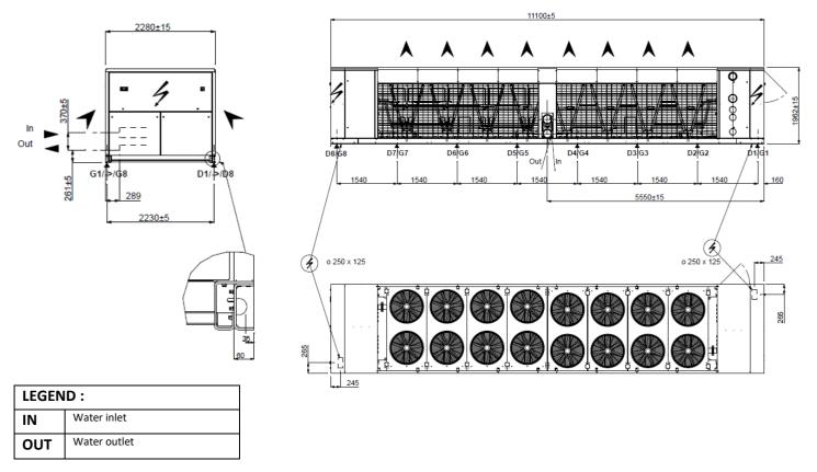
Note: In case of single main power connection (option), main power supply and disconnect switch are located at the right side of the unit.
