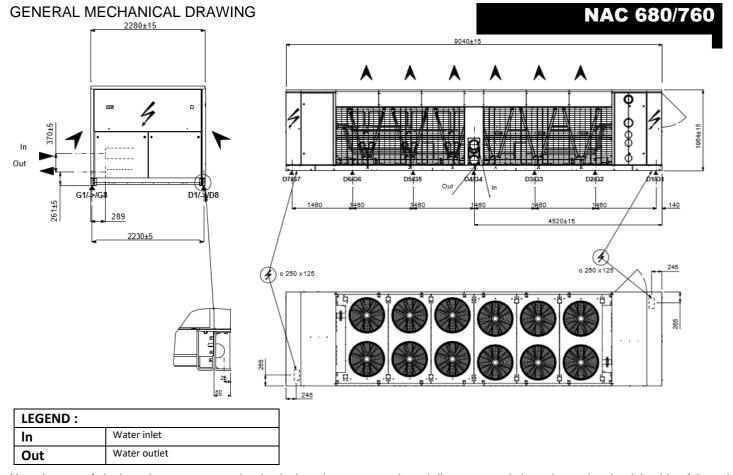
Note: In case of single main power connection (option), main power supply and disconnect switch are located at the right side of the unit.
