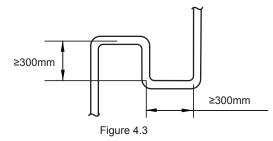
The piping length and level difference requirements that apply are summarized in Table 4.1 and are fully described as follows.
