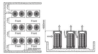
If obstacles are around the outdoor unit, they must be 800mm below the top of the outdoor unit. Otherwise, an mechanical exhaust device must be added.
