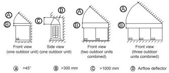
If the particular circumstances of an installation require a unit to be placed closer to a wall. Depending on the height of adjacent walls relative to the height of the units, ducting may be required to ensure proper air discharge. In the situation depicted, the vertical section of ducting should be at least H-h high. If the outdoor unit needs ducting and the static pressure is more than 20Pa, the units should be customized for the corresponding static pressure.
