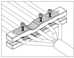
Then, use 3 pieces of M4\*30mm screws to secure the upper cover. At the same time, be careful not to screw it too tight. If you use excessive force to twist to the end, you may destroy the protection layer of the power cable.
