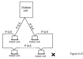
After the last indoor unit, the communication wiring should not route back to the outdoor unit as this will form a closed loop.
