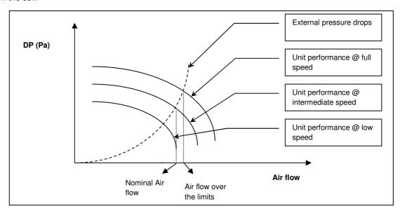
The fan speed has to be selected according to the enclosed table.
