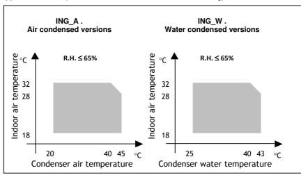
Applications with an external air temperature below 20°C, require a condensing control to ensure enough pressure drops through the expansion valve. Temperatures below -20° and down to -40°C require a flooding device in order to flood the condenser internal surface and get the right condensing T, even in case of strong and cold winds.
