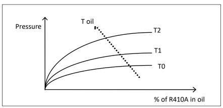
The diagram above illustrates a specific property of gases (Charles' Law), which are more soluble in liquids as the pressure increases but less soluble as the temperature increases: if the oil in the sump is held at a constant pressure, an increase in temperature will significantly reduce the amount of refrigerant dissolved in it, thus ensuring that the desired lubricating function is maintained.
