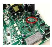
3. Check the power supply for the compressor inverter module, port CN211 on filter board, the normal voltage should be DC310V; Check the single phase bridge and fuse on filter board; check the connection cable from ODU main PCB port CN4 to filter board port CN8 which is 12V DC power control port.
