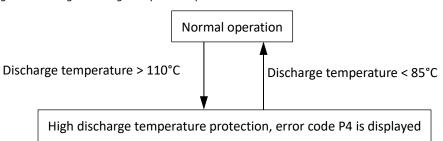
When the discharge temperature rises above 110°C the system displays P4 protection and the unit stops running. When the discharge temperature drops below 85°C, the compressor enters re-start control.
