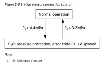
When the discharge pressure rises above 4.4MPa the system displays P1 protection and the unit stops running. When the discharge pressure drops below 3.2MPa, the compressor enters re-start control.
