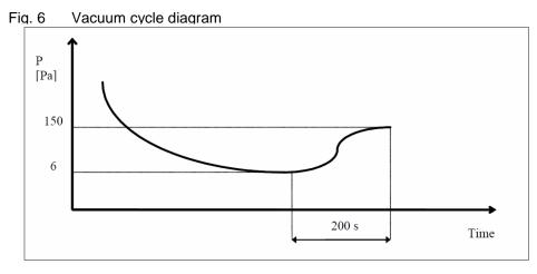
The Fig. 6 represents a vacuum cycle and an optimal subsequent pressure rise for the refrigeration devices we manufacture. As a rule, if there is suspicion of an extensive presence of humidity throughout the circuit or system as a whole, the vacuum must be "broken" with anhydrous nitrogen and then the steps must be
