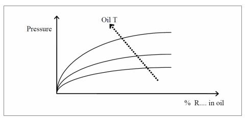
The diagram in Fig. 9 illustrates a specific property of gases (Charles' Law), which are more soluble in liquids as the pressure increases but less soluble as the temperature increases: if the oil in the sump is held at a constant pressure, an increase in temperature will significantly reduce the amount of refrigerant dissolved in it, thus ensuring that the desired lubricating function is maintained.
