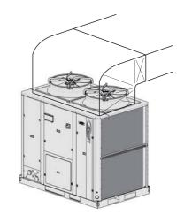
In units 1003-2104 SM, if only one duct is going to be installed, a regulated pressure damper should be installed for each fan, to avoid air by-pass through the fan if it has stopped.
