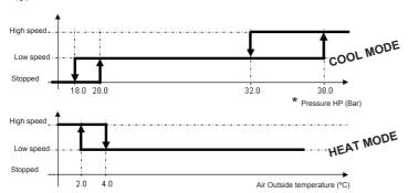
In this mode, the fan capacity is limit according to the sound level desired. For fan using low / high speed the high speed is locked.
