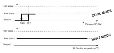
This mode is similar to the "Quiet" mode except that the fan speed limit or the high speed is never unlocked.
