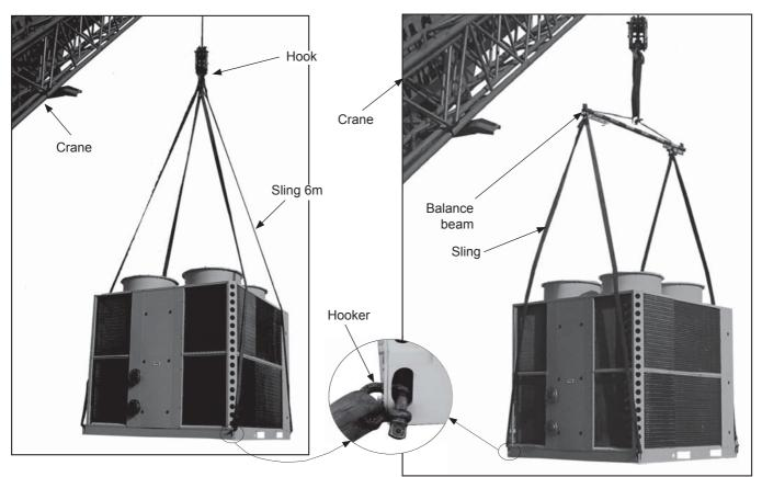
**NOTE:** Use slingers of 6 m with the hook in order to prevent pressure on the top of the unit because it can be damaged. Whenever it is possible, use balance beam.
