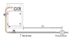
A pressure gauge must always be installed upstream and downstream of the main gas supply line visible with a scale of [0-60] mbar (0.06 bar) in order to verify any difference in upstream and downstream pressure and therefore the flow rate of the entire network.
