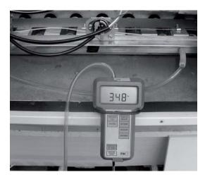
• after the adjustment of the low heat, re-verify the high heat, re-position the stoppers and close the pressure ports.
