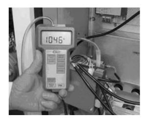
The out pressure must be measured on the pressure tap located on the gas injector support bar to avoid the pressure drop due to the elbow after the valve
