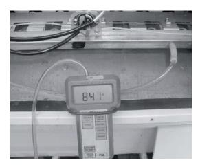
place the tube of the "accurate" manometer to the out port on the gas injector support bar after having loosened the screw by one turn.
