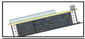
After levelling the frame, secure the adjustable returns on the trimmer.
