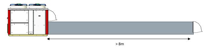
It is recommended to sheath the exhaust air by at least 8m (according to local regulations) to escape the fresh air inlet when the input-output are on the same side.
