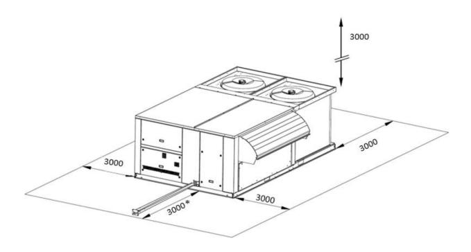
\*: Add 1000 mm if the units are equipped with gas burner
