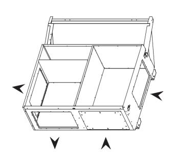
WARNING: a multidirectionnal flowcurb and horizontal extraction flowcurb must be secured to the ground using existing fixing holes on the frame.
