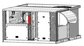
Drill the sheet metal to the diameter of the cable glands It is recommended to use only one cable per cable gland
