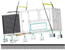
Place the 4 side feet and 4 corner feet (supplied loose) in place of the transport feet and sleeves and tighten moderately with screws and washers.
