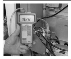
**HIGH HEAT INJECTION PRESSURE CHECKS** Check and adjust if necessary the valve OUTLET pressure.
