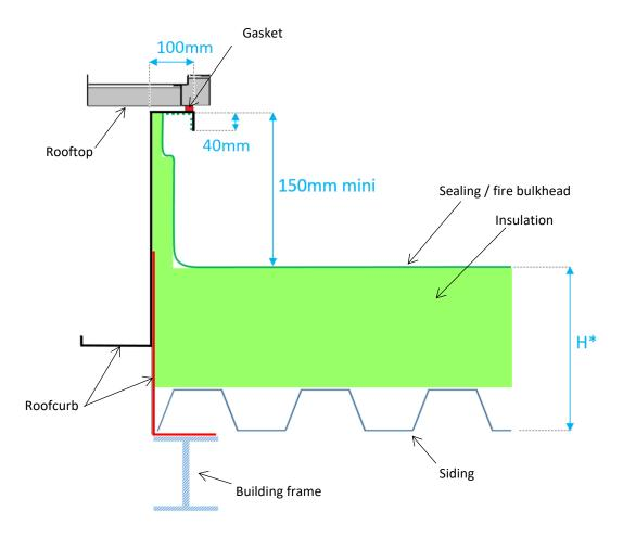
\* Check that the roofcurb height is enough to respect a sealing height of 150mm minimum (French DTU 43.3) considering the building specifications: geometry of the roof, material and thickness of the insulations and other protection layers, slope of the roof...).
