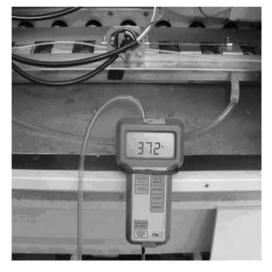
After the adjustment of the low heat, re-verify the high heat, re-position the stoppers and close the pressure ports Pressure adjustments table for each type of gas (mbar)
