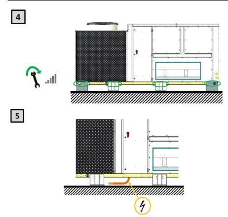
Complete the tightening of the feet screws.
