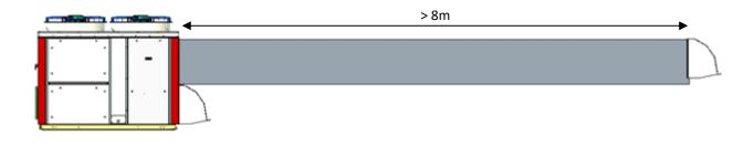
It is recommended to sheath the exhaust air by at least 8m (according to local regulations) to escape the fresh air inlet when the input-output are on the same side.
