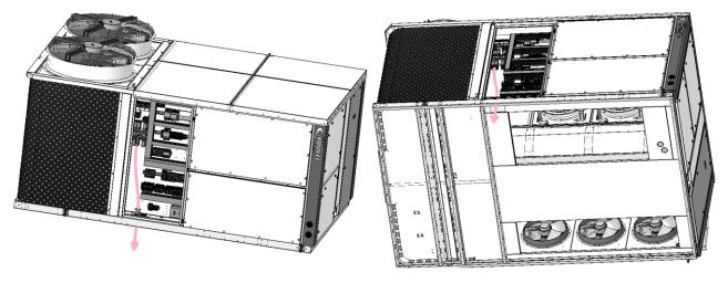
Pass through the cable glands at the bottom of the electrical box. Drill through the insulation if necessary.
