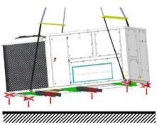
First, remove the 4 transport feet and the 2 sheath when the Flexair unit is lifted.
