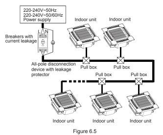
Refer to Tables 6.1 and 6.2 for the specifications of the power cord and communication wire. A wiring capacity that is too small will cause the electrical wiring to become too hot, and lead to accidents when the unit burns and becomes damaged.
